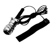
New infra-red, photoelectric plethysmograph records changes in pulsatile blood flow from fingers, toes, ear, forehead, etc. Miniature transducer attaches with velcro strap (supplied) or electrode type adhesive collars. Matched optics together with a unique two-stage IR-filter reduce the effects of ambient light and patient motion.
