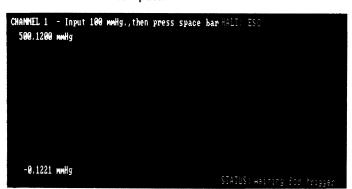
Calibration of the system, using Gould's Medical Instrumentation Amplifiers, is as easy as pressing the space bar. Gould's exclusive shunt-cal system assures positive, accurate calibration by electronically simulating a 100 mm Hg pressure load using transducer and amplifier circuitry. The scaled output from the Gould's amplifiers means the computer input is not affected by changes in the full scale setting of the amplifier.
