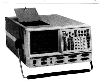
The K450 belongs to the new generation of logic analyzers. Its feature set is optimized to solve not only routine problems, but also those complex and elusive failures which occur intermittently. Its powerful features, combined with easy setups, make this Logic Analyzer an indispensable tool for hardware and hardware/software engineers who are working with custom digital boards, bit-slice systems, ECL state machines, gate ar-
