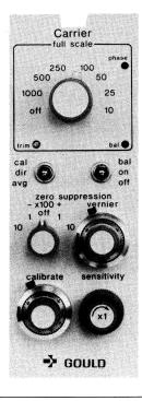
The Gould Carrier Amplifier measures pressures, forces, and displacement with unprecedented ease. By replacing separate, interactive R and C balance controls with electronic auto balance, as well as auto phase lock of excitation and signal, it provides features never before available to users of AC excited transducers. Eliminates time-consuming setup or phase errors. Just flip a switch and it's balanced. It works equally well with LVDT, variable reluctance, and strain gage transducers.
