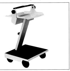
Gould's mobile Instrument Cart is specifically designed for the K-XXX series Logic Analyzer family. The cart is constructed of sheet steel that is finished with a Gould Gray paint. The base has a black rubber mat on the surface, and a 1.5 in. black nylon protective bumper strip. The 5 in. caster system, having swivel front casters and rigid rear casters, makes the cart especially
