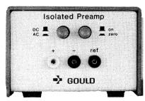
This 10-kHz Amplifier provides the high impedance inputs, high gain, and low noise characteristics required for recording bioelectric potentials including HIS Bundle, EMG, EOG, ENG, and ECG. One-mV or 50- $\mu$ V cal signals and a full range of high-pass and low-pass filters permit the Amplifier to easily reproduce the most demanding bioelectric signal.
