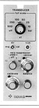
The Gould Transducer Amplifier is a precision signal conditioner for measuring pressure, force, or position. It provides ultra-stable excitation for DC strain gage transducers while providing for plug-in bridge completion resistors.
