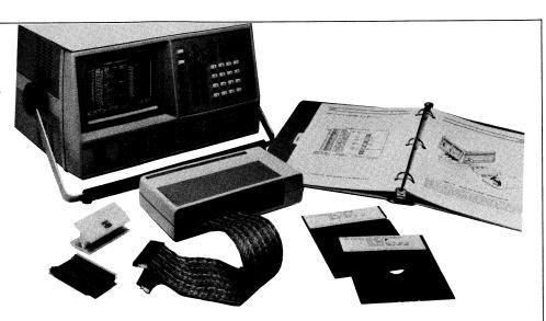
Microprocessor Analysis Packages (MAPs) provide complete interfacing and disassembly for most of the popular microprocessors in use today. In addition, a User-Definable Disassembler and Interface Adapter will support any additional standard or custom processors.
