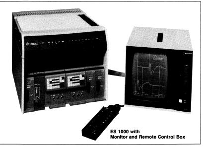
The Gould ES 1000 is a modular, highly versatile electrostatic array recording system. Its modular design allows you to configure a solution to meet current needs and to expand for future needs. The fixed, no-inertia electrostatic writing head has no moving parts, increasing reliability.
