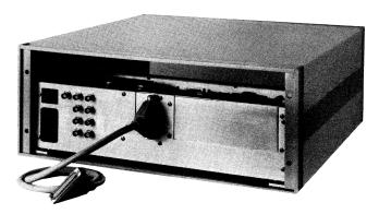
Back panel of 5900 Cage with 3000-to-5900 Connection Cable.
